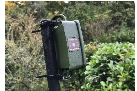
Image 1: Correct placement of the bat detector
