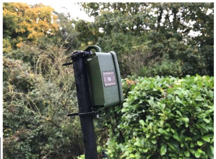
Image 1: The detector mounted to the top of the pole horizontally with the microphone pointing to the side.
