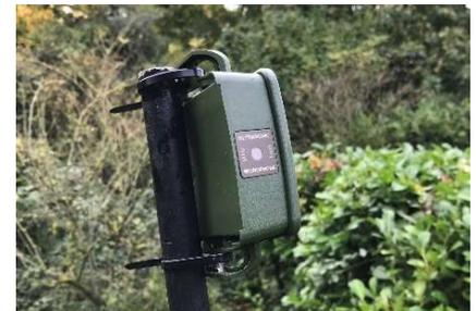
Image 1: Correct placement of the bat detector
